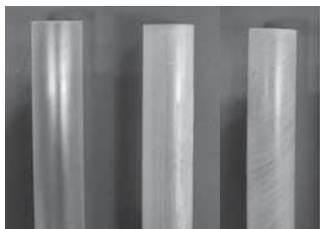
Fig(1)Left:[No processing] Center:[linear riblet] Right:[Spiral riblet]
