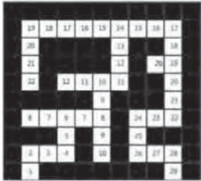
Figure 1 Flood Fill Algorithm (Maze Robot)
