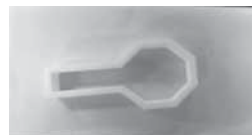
Figure 2. Spoon mold made with a 3D printer
