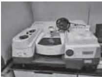
Fig.7.Fourier-transform infrared spectroscopy (FTIR)
