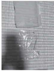
Fig. 3 Agar plastic produced in Container 2
