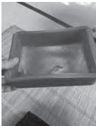
Fig. 11 Distorted 3D printed container
