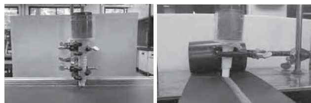
Figure 3. Writing simulation by pressing the chalk down with weights
